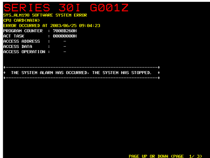
Example of system alarm screen
